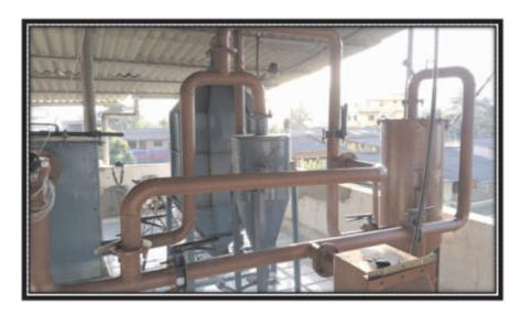
The measurements are made at the outlet of the water scrubber.
