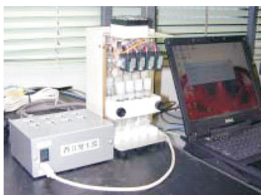
Fig.4 picture of perfume emitting device connected to a PC developed at Fukui national college of technology.
